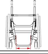
Note: higher than 20" Front STFH will reduce the footrest width up to 1" with a 2" taper
