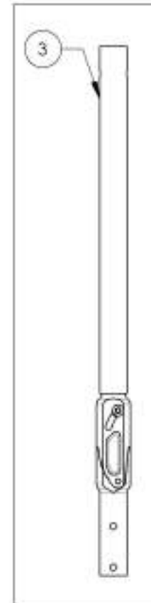
9001249 Back Cane - Carbon Fiber, Angle adjustable, Straight, 18-21 in
