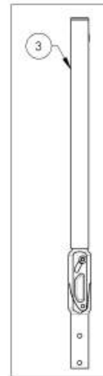
9001262 Back Cane - Carbon Fiber, Angle adjustable, Fixed 18 in
