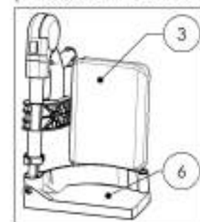
9002484 Complete Elevating Legrest - Swing-In/Swing-Out, Right + Composite Footplate (Wheelchair Width: 19 in +)
