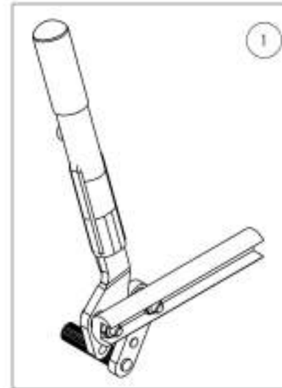
Default Wheel Lock - Pull to Lock, Extended Rail, 6 in Removable Extension Handle, Right
