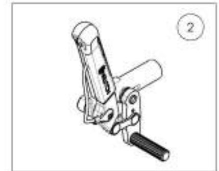
9002219 Wheel Lock - Newton Spring Loaded Push to lock, 6 in Removable Extension Handle
