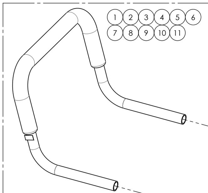
UTILISER LE MANCHON #0032001A-00 SI LA POIGNÉE DE POUSETTE (#0051523A À #0051533A) SERA INSTALLÉE AVEC LES MONTANTS DE DOSSIER ALUMINIUM DROIT AVEC POIGNÉE INTÉGRÉE (#9003298A OU #9003299A)
