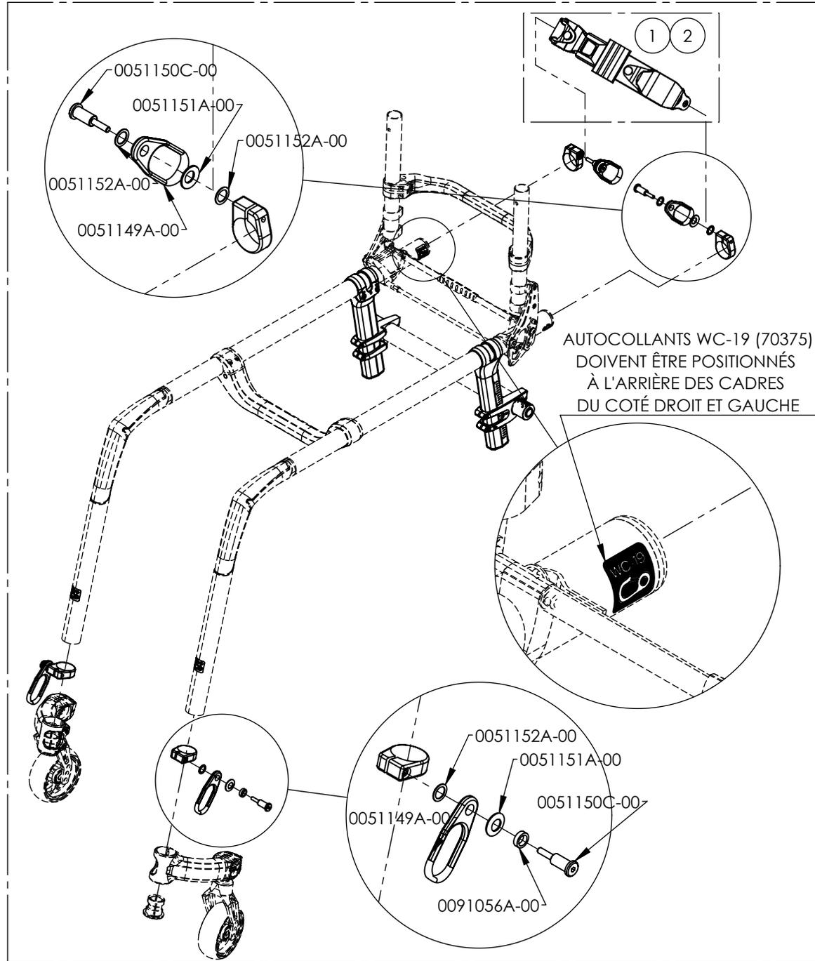
LA MISE À NIVEAU WC-19 DOIT ÊTRE SÉLECTIONNÉE AU MOMENT DE LA COMMANDE DU FAUTEUIL (DES AJUSTEMENTS SPÉCIFIQUES SONT REQUIS)
