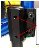
Unoccupied transport anchors installation (screws #90659)
