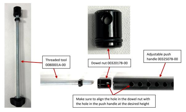
• The adjustable push handle can adjust 3". Each hole is 1/2" apart.
